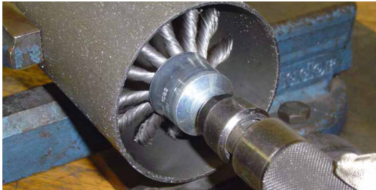
Opening of the end brushes depending on the RPM
