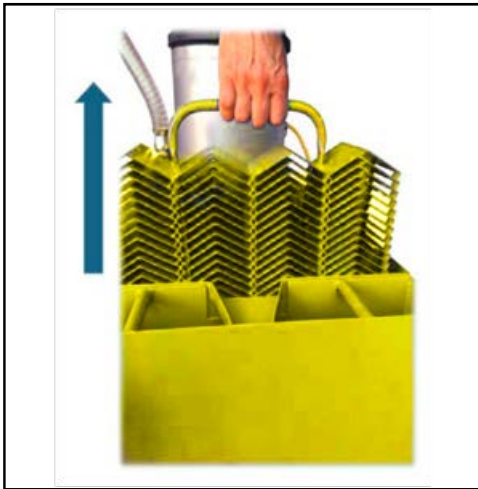
Figure 5: Removal of the oblique plate filter block
