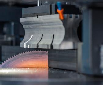
Clamping, sawing, reverse motion, opening – at the touch of a button
