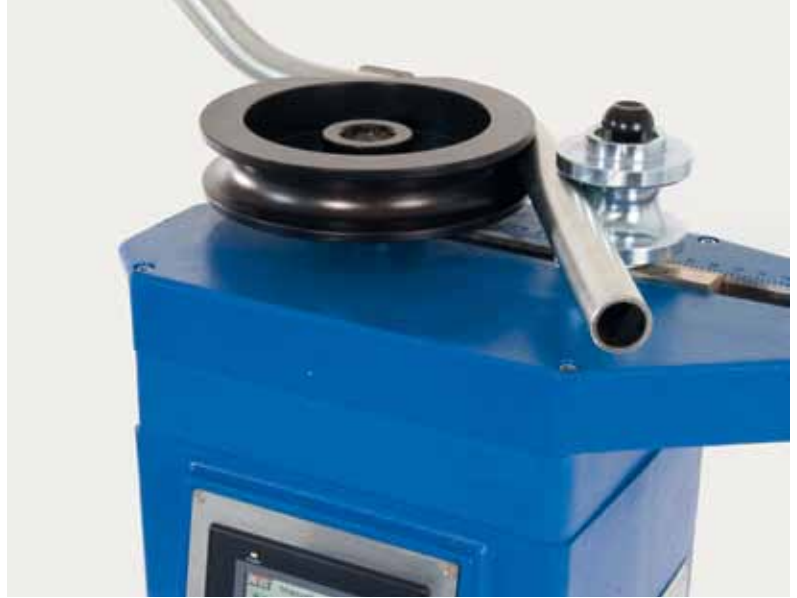
Bending with counter roller for thick-walled tube
