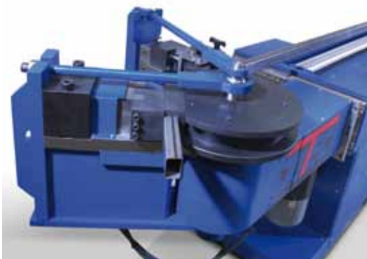
Mandrel bending device 8000 with bending tool for square tube 60x40 mm
