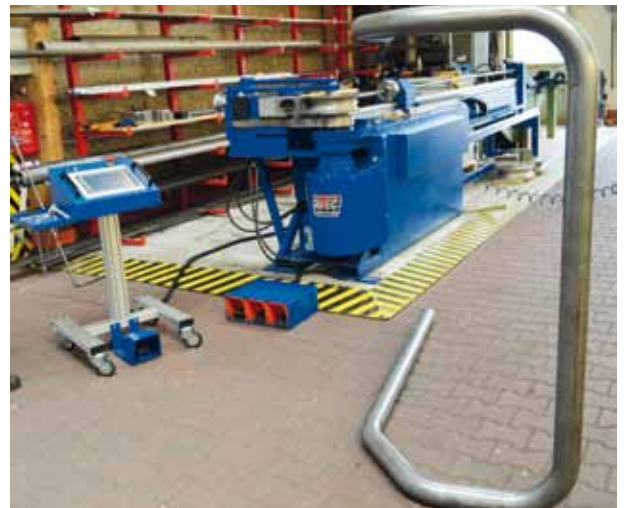
Bending capacity up to 100 mm possible with mandrel bending device 9000
