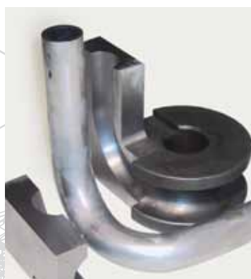
Mandrel bending tool bend-to-bend ( e.g. door handle )
