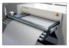
The material is fed smoothly into the machine where the integrated straightening results in completely flat sheets with no pause marring.
