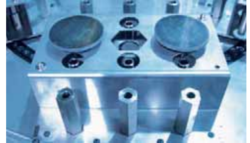
Multi-pallet attachment for a family of parts
