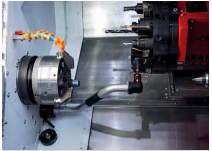
Tool measurement. The optional tool measurement sensor mounted in the work area enables quick and precise measurement of the tools within the machine. It is manually mounted below the main spindle. After use, it is placed in a storage area at the left machine cover.
