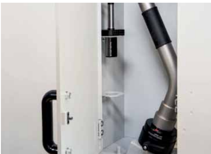
Tool measurement sensor storage niche. Protected storage area for the tool measurement sensor and setting gauge.
