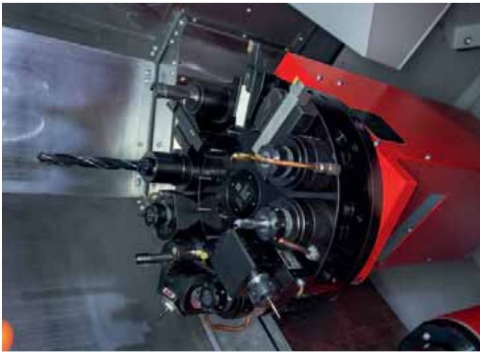
Axial tool turret for the tailstock version. Quick 12-fold servo turret with very short indexing times for standardised VDI30 or VDI40 tools. All stations can include driven tool holders for drilling, milling or thread-cutting operations. The operator can influence the swing speed at any time.
