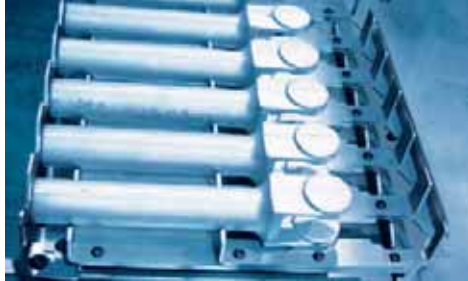
6-station pallet attachment for articulated brackets
