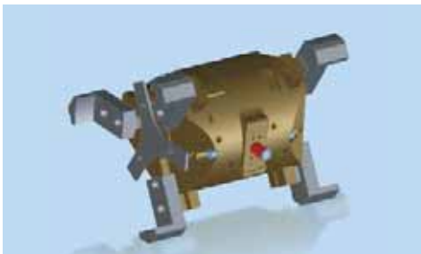
2 x 3-jaw double gripper head
