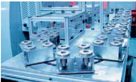
4-station pallet attachment for valve caps
