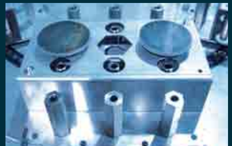
Multi-pallet attachment for a family of parts
