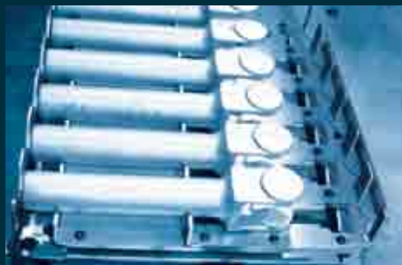
6-station pallet attachment for articulated brackets
