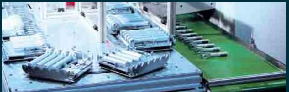
20-station pallet magazine with customer-specific pallets
