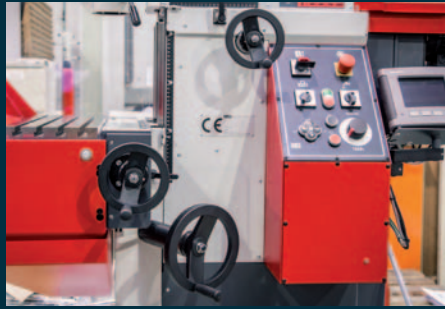
Safety handwheels (X/Y). Ergonomically placed handwheels ensure easy and safe handling in all three axes.
