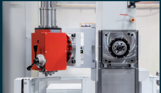
Swiveling device. Swivel-mounted vertical milling head. Controlled by end switch.
