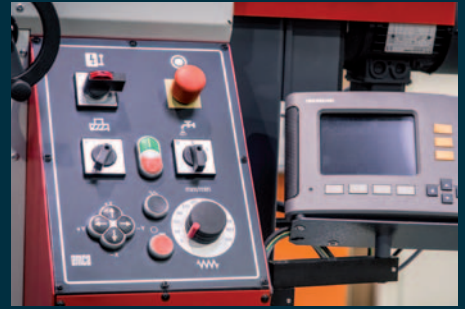
Control panel. Control panel with ergonomically designed keypad and a swivel mounted position display for easy operation.
