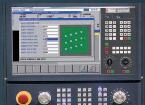
The change to a different control system is carried out within a minute by calling up the respective software.
