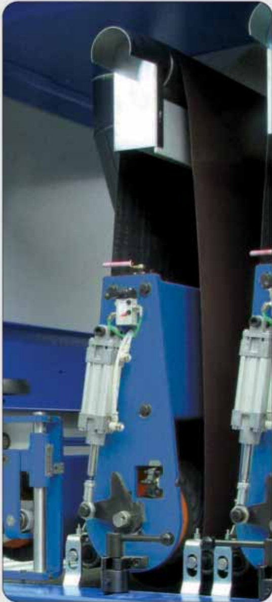
Cylinder unit - Pneumatic Grit-set with 6 position revolver to quickly compensate the thickness difference of the various types of abrasive belts.
