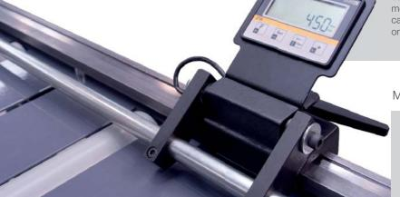
Without additional electric power supply, with a durable battery, the digital measuring stop MRA offers precision measurement along the entire length. The stop carriage is adjusted manually, and its position is shown on a digital display with the accuracy of 0.1 mm.
