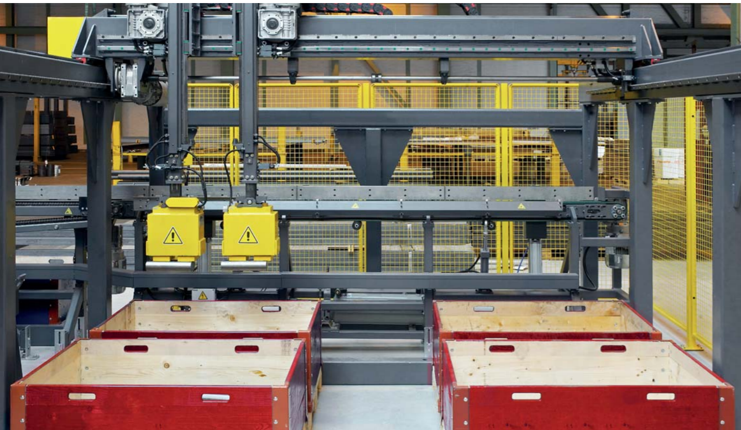
Custom-made solution with a Cartesian robot
