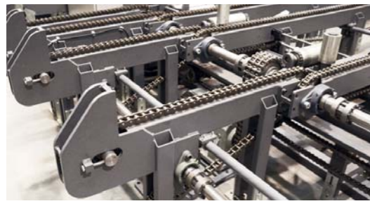
Load- and wear-resistant transverse feeding units on the inlet side with high-efficiency drives
