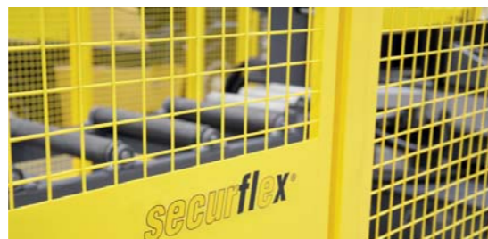
SECURFLEX safety system, combined with grid elements and laser-light barriers
