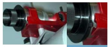
'cam dogs' aligns with the mating 'notch' in the fixture.
