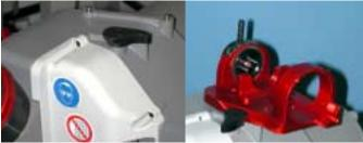
Fixture. Now would be a great time to determine the point angle of the drill that is to be sharpened and adjust both the sharpening fixture and alignment to that point angle. The Sharpening fixture is adjusted by pulling the red lever towards (counter clockwise) the operator and sliding the fixture to
