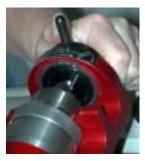
the operator will increase the relief. Placing the pin at the midway point on the decal is a good starting place for 118° drills. For 135°-150° drills start with the alignment 2 marks towards the operator. You can set the alignment at any setting necessary to achieve the amount of relief desired.
