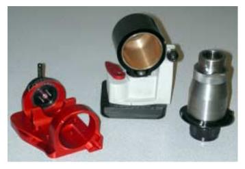
and SA16500TA Large Drill Chuck. By now you are familiar with the 'quick disconnect' feature of your **XT-3000**. Start by placing the Large Drill Alignment on the top of your **XT-3000**. Rotate the 'Docking Lever' clockwise to securely lock the fixture in place. In a similar manner, remove your current sharpening fixture and replace it with the Large Drill Sharpening
